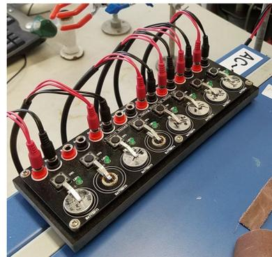
Prototypes of "coin cell" batteries that integrate the polymer binder technology are tested in Dr. Yu Zhu's lab
